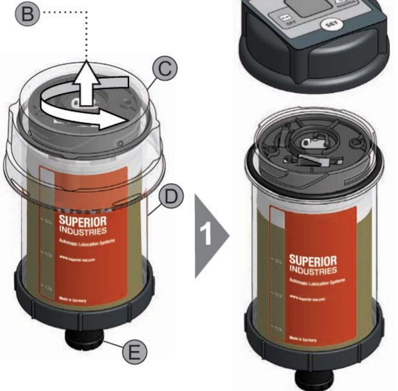
Rotate the cap a 1/4 turn, clockwise, until the corner of the cap is in line with the arrow (see below).
