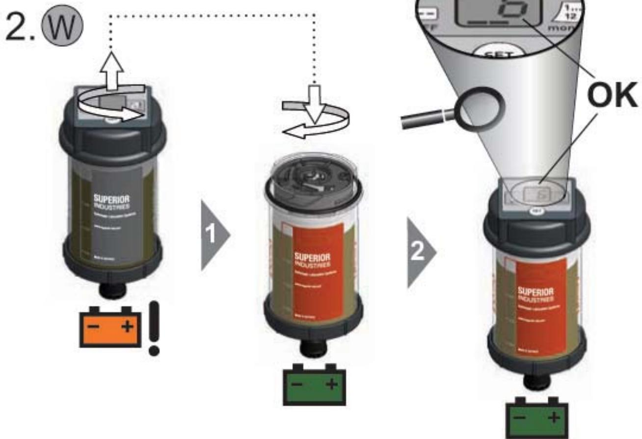
12 different dispensing rates are available (1-12). 1 means that the contents of the cartridge will empty over a one month period, (approximately 4.2cc/day for one 130cc cartridge OR 8.4cc/day for two cartridges on one grease zerk.) 2 means the same cartridge will empty over a two month period, (approximately 2.1cc/day for a 130cc cartridge OR 4.2 cc/day for two cartridges on one grease zerk.) etc...
