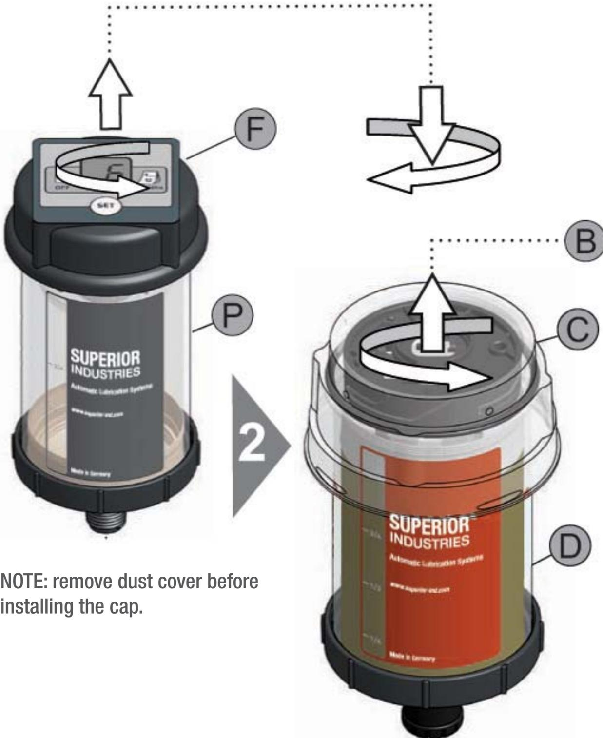
NOTE: remove dust cover before installing the cap.
